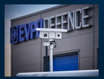
The monitoring device can be installed on any type of vehicle which has a sufficient space needed for installation. The basic outline of the vehicle remains unchanged even after complete modification. Installation is solved through the box body, where the special monitoring system is built-in, completed with thermal vision camera.
